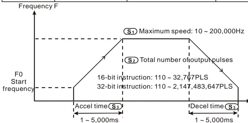
3. The acceleration/deceleration of EH/EH2/SV/EH3/SV2 series MPU is based on the number of pulses. If the output cannot reach the maximum acceleration frequency within the acceleration/deceleration time offered, the instruction will automatically adjust the acceleration/deceleration time and the maximum frequency.
