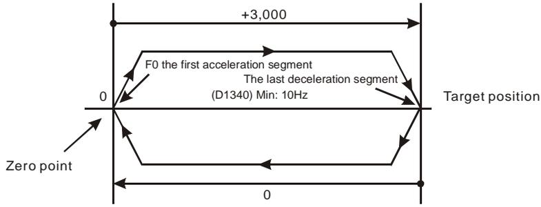
b) Settings of absolute positioning and the acceleration/deceleration speed:
