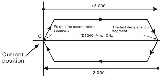
b) Settings of relative positioning and the acceleration/deceleration speed:
