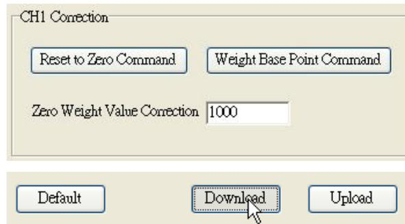
8. Click “Weight Base Point Command” to set up the weight base point. Now, the weight at CH1 is 1,000kg.
