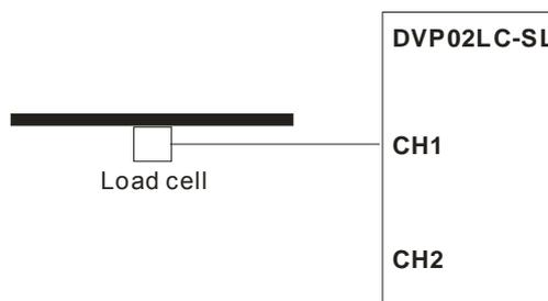
3. Set up every parameter and eigenvalue according to the actual measuring requirements and specifications of the load cell. In this example, we use the default settings of all parameters.
