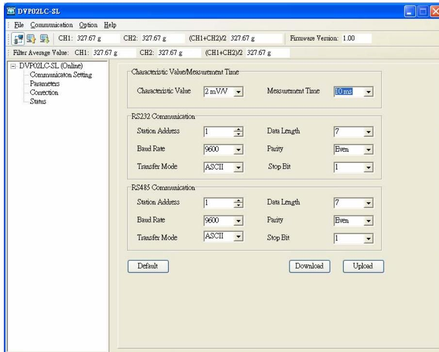
2. Set up also the average times and maximum weight. Due to that we connect two load cells in parallel and connect them to a single channel here, we have to disable CH2.
