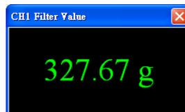
Note: When the filtering function is not enabled, the window for the filter average value will display “32767”. Once the filtering function is enabled, the average times have to be > 30, and the filter percentage has to be set.
