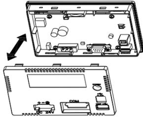
Step 3: Complete the following steps, ① and ② to replace a battery.
