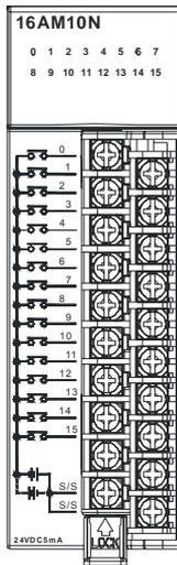
5. Digital output module (16 outputs)
