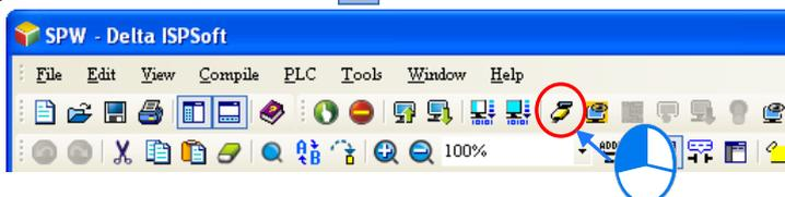
Not only the logic program, but also the information related to the devices is monitored. (If the data type is a Boolean value, the state of the device is represented by green (ON) or white (OFF). If the data type is not a Boolean value, the value in the device is shown.)
