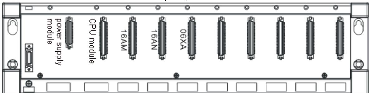
Connect the module to the connector on the backplane, make sure that the module is installed on the backplane properly, and tighten the screw.
