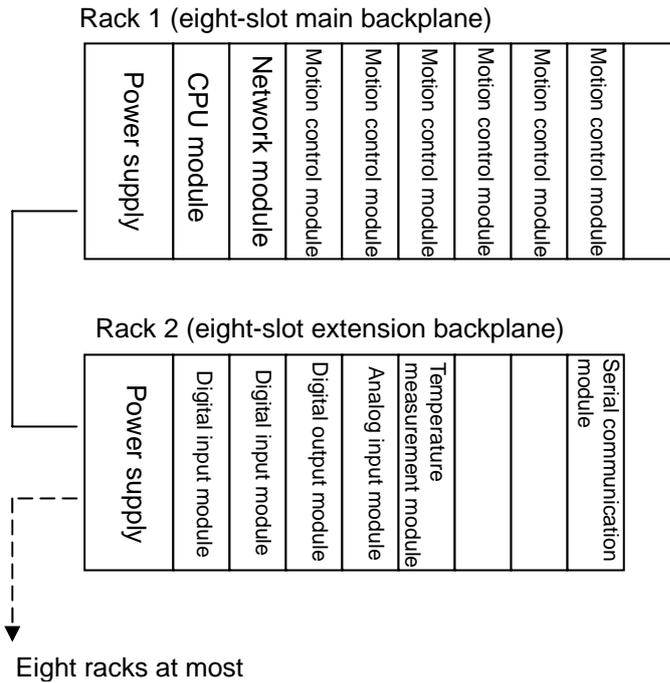
Note: Owing to the consideration to the data transmission speed, the motion control modules and the network modules (exclusive of the serial communication modules) have to be installed with the CPU module on the same backplane. Otherwise, the system can not operate properly.
