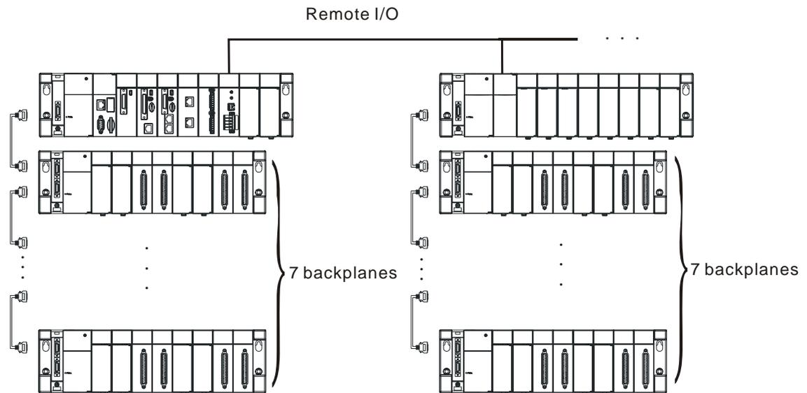
Note: Users are provided with the special cables to connect the extension backplanes. The length of a special cable can be up to 100 meters. They are also provided with the fiber cables which are used with the special adapters. The length of a fiber cable can be up to 2 kilometers.
