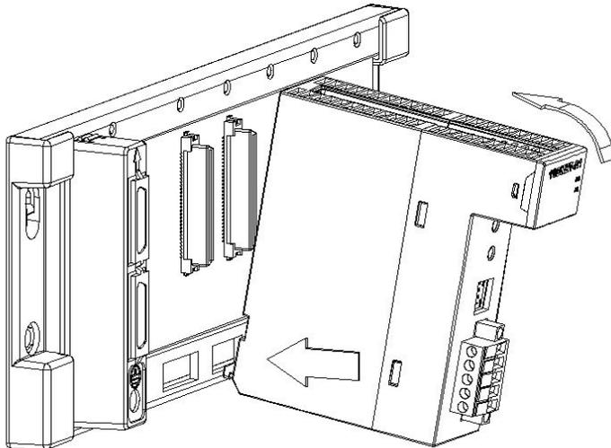
3. Tighten the screw on the module.
