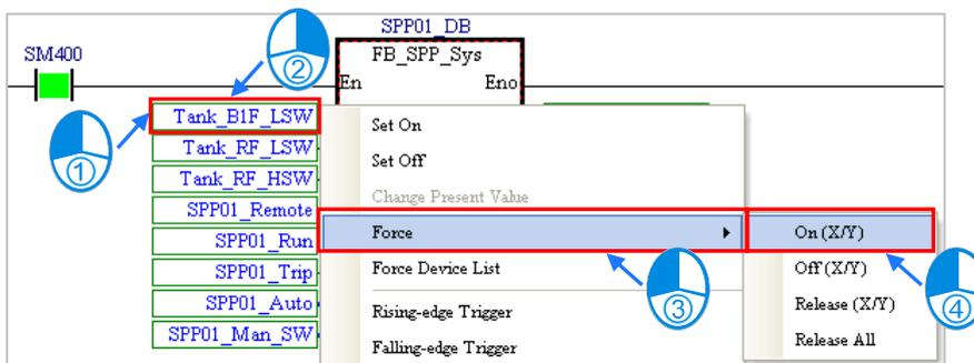
The value in the device is altered, and a lock symbol indicating that the device is forced ON appears.
