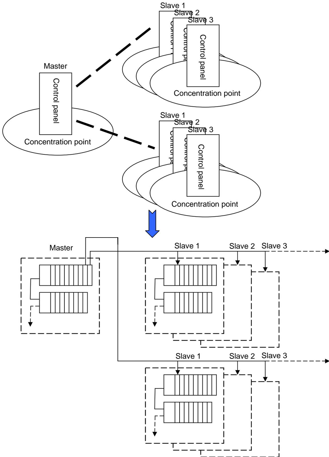
Note: The remote masters in DeviceNet are the network modules. They have to be installed with the CPU modules on the same backplane. A CPU module can support eight masters, and a master can be connected to sixty-three slaves. Besides, a slave can be connected to seven
