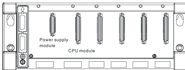
The common framework of the AH500 system (for original equipment manufacturers):
