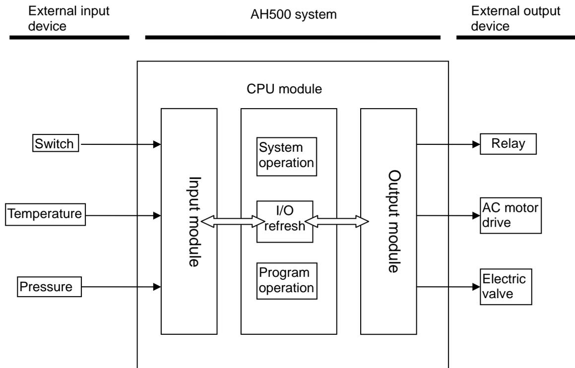
The operation of the CPU module is illustrated above. The system procedures related to the initialization, the diagnosis, and the communication, and the program procedures related to the external interrupts and timed interrupts are simplified. Users can refer to other manuals for more information. The operation of the CPU module is described below.
